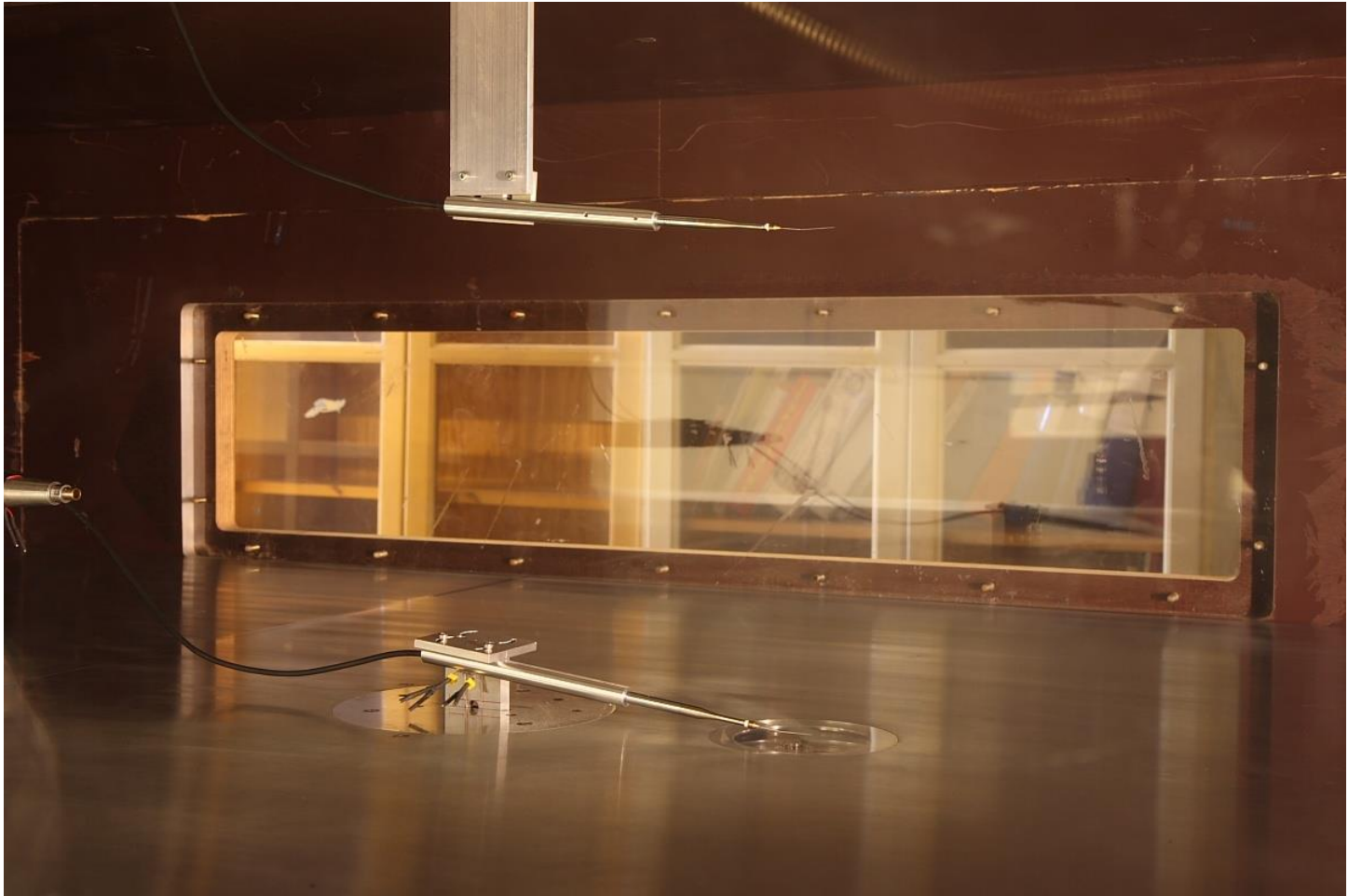
Pressure probe setting in KTH wind tunnel
